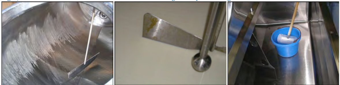
Fig. 48 Left-milk stone in tank; centre-biofilm on agitator paddle; right-clean tank
