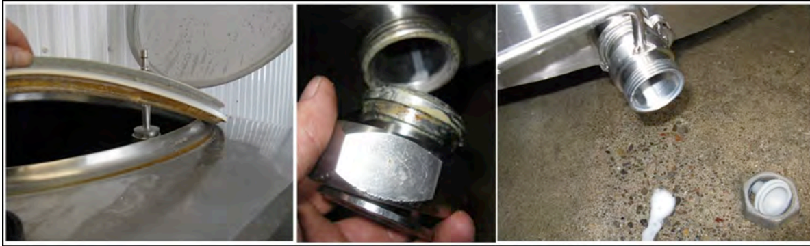
Fig. 49 Milk tank equipment needs to be inspected and cleaned after every pick-up
