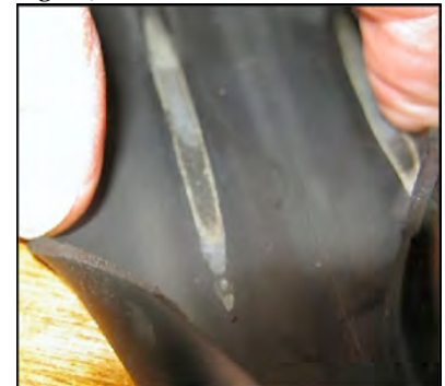
Fig. 24 Liner cracks with bacteria
