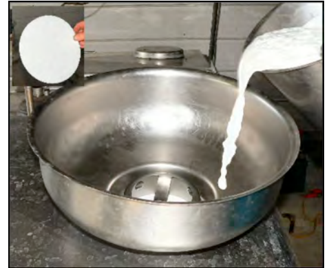
Fig. 42 Milk poured through strainer fitted with filter. System used with hand-milking or bucket.
