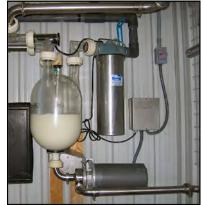
Fig. 40 Receiver jar with milk pump and trap
