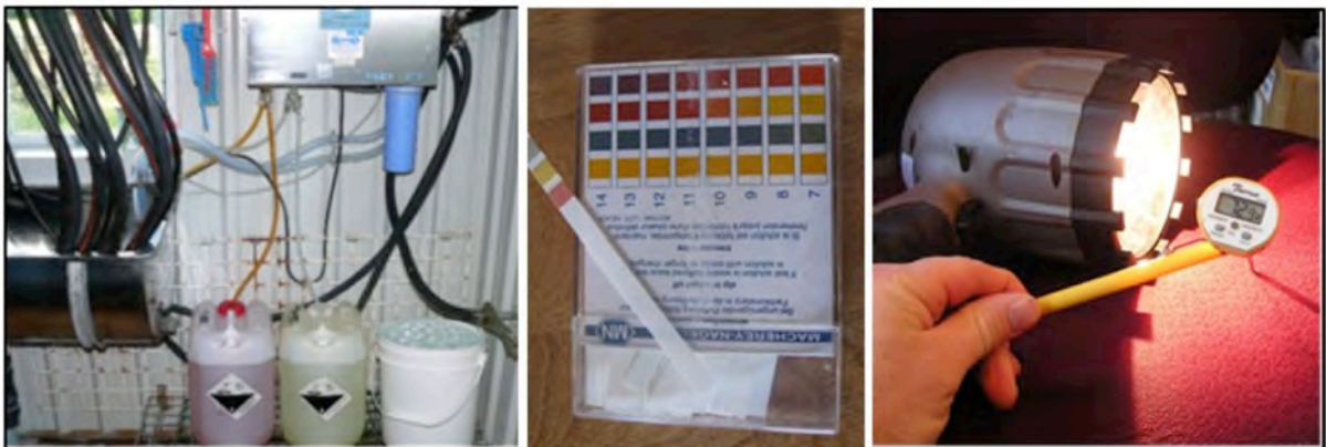
Fig. 30 Left - verify cleaners used correctly; Middle - pH paper to check acidity / alkalinity; Right - thermometer and strong flashlight
